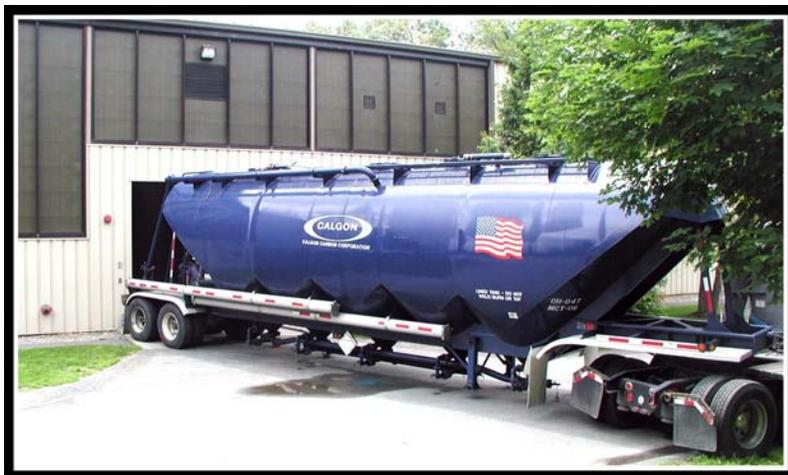
Delivery of carbon for groundwater treatment units
